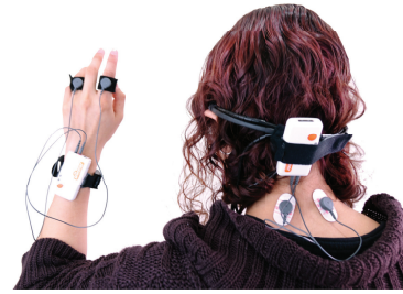
Fig. 1. Wearables to gather data. From left to right, the usage of the Shimmer3 GSR on the hand, and the Shimmer3 GSR integrated on an EMG wearable to measure skin conductance from the neck.
